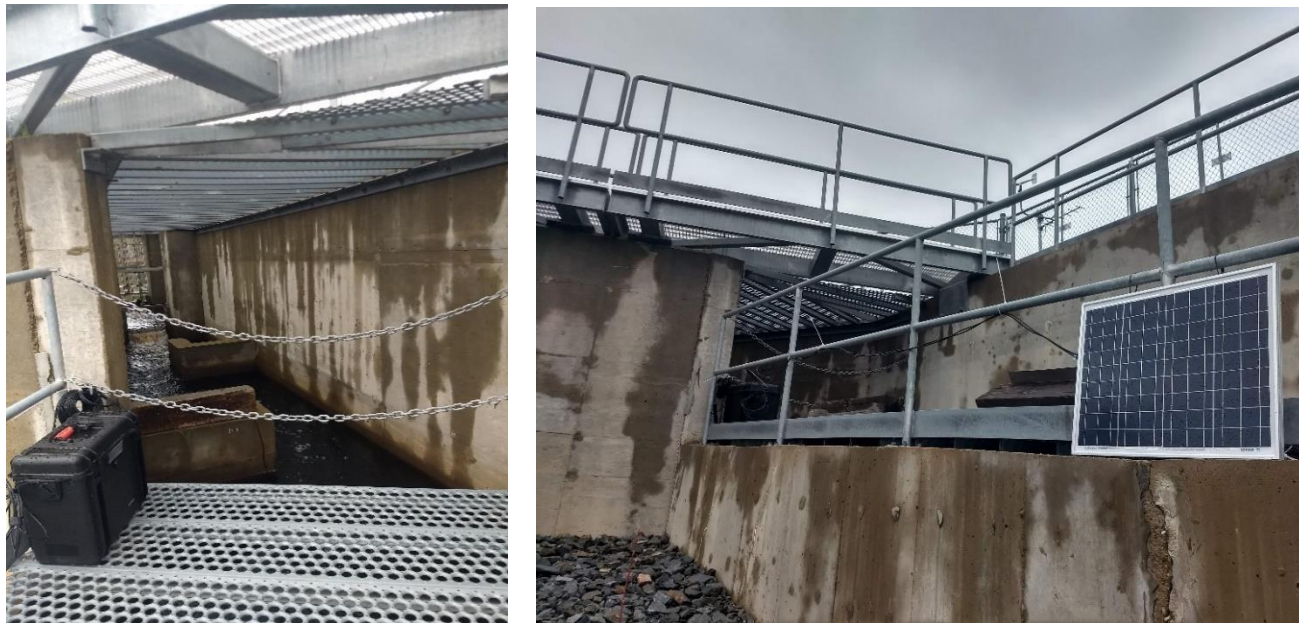
Figure 4. The upper section of the Hebb Dam Fish Passage Facility showing the placement of the camera and accessories. Left: the camera is placed underwater, adjacent to the first concrete baffle. The case contains the control panel for the camera. Right: the solar panel used to power the Biotactic Bravo Generation 2 camera.
