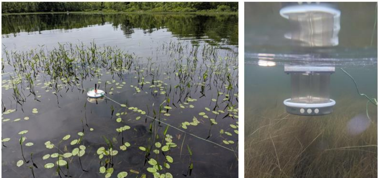
Figure 5. Above- and below-water view of a deployed light trap. Photos were captured in 2020.
