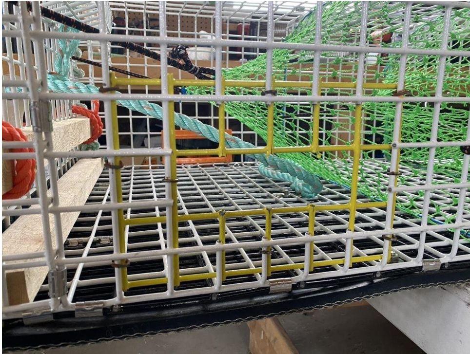
Figure 15. Yellow escape panel on white lobster trap attached with iron hog rings.
