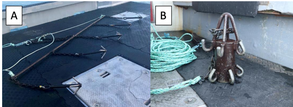
Figure 3. Grapples used in the 2022 season for gear retrieval. A. span drag, B. cylinder block grapple.
