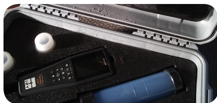
Figure 3: A YSI sonde with built-in sensors used by Sherbrooke Lake volunteers to monitor the physical properties of the water.
